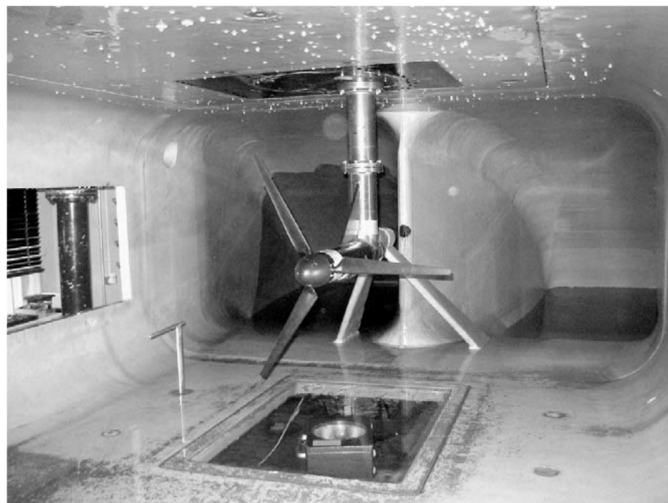
FIGURE 3.6: PHOTOGRAPH OF EXPERIMENTAL SETUP IN THE CAVITATION TUNNEL (BAHAJ ET AL. , 2007A)
