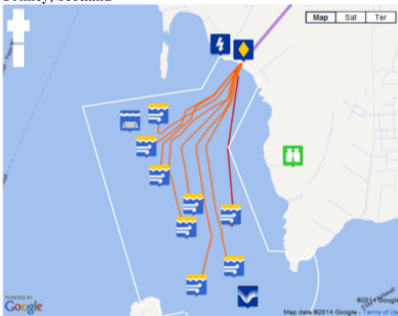
Fig.1.2: Layout of the EMEC tidal energy test site at the Fall of Warness, Orkney, Scotland
