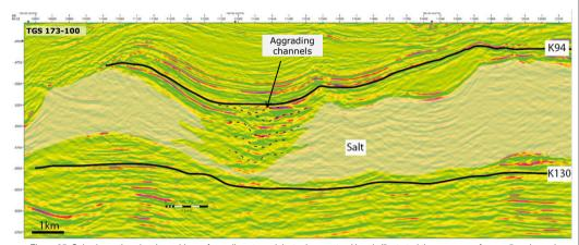
Figure 35: Seismic section showing evidence for sediment conduits to deep-water. Here is illustrated the presence of aggrading channels within a small mini basin on top of the salt canopy. It is to be noted that here again the K101 is absent.
