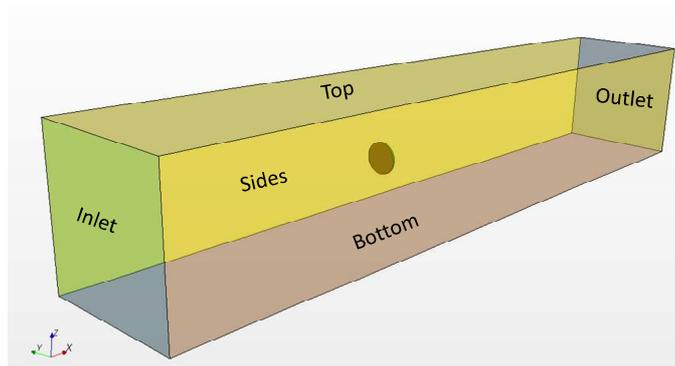
Figure 4-8: Closed channel CFD model of flume tank
