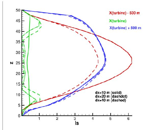
Figure 5-5: Length scale (m) using  $k$ - $\epsilon$  turbulence closure.Table 5-5 - convergence for  $A_v = 0.1 \text{ m/s}^2$
