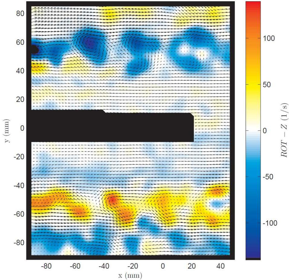
Figure 3-11: Large vortical structures shed from the disc edges were evident in the experimental flows.
