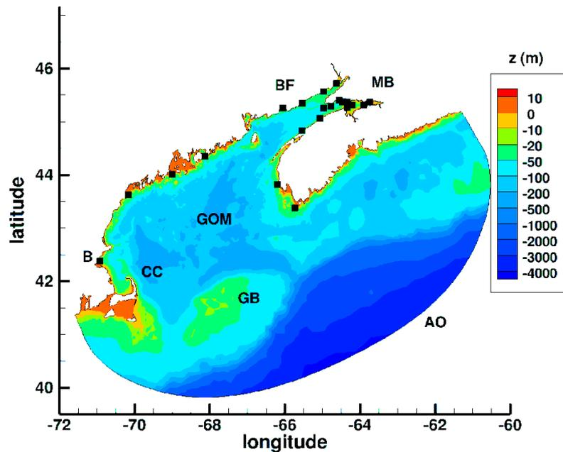
Figure 6-1: Geometry and bathymetry of Bay of Fundy. Sea level observation sites are denoted with a  $\square$ . AO is Atlantic Ocean, GOM is Gulf of Maine, BF is Bay of Fundy, MB is Minas Basin, GB is Georges Bank, B is Boston, and CC is Cape Cod.
