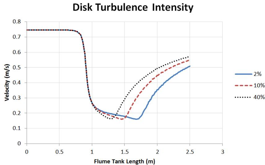
Figure 4-11: Centre-line velocities for different disk turbulent intensities
