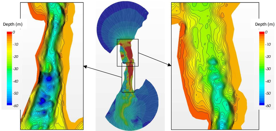
Figure 7-14: Depth Contours for Petit Passage
