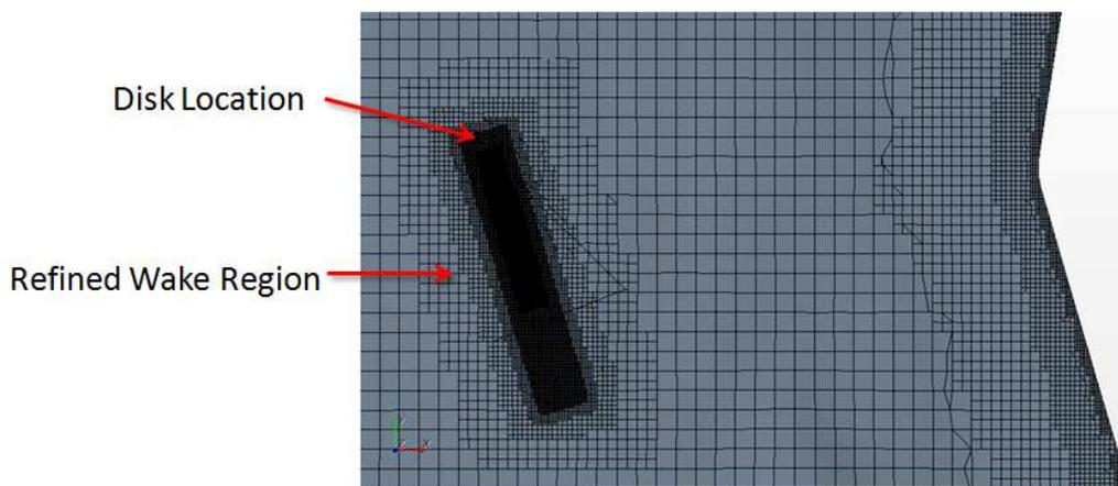
Figure 7-19: Top view of Petit Passage mesh with local mesh refinement around a porous disk. The mesh shown was for the North-to-South flow case.
