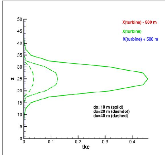
Figure 5-3: Turbulent kinetic energy using *k-e* turbulence closure.
