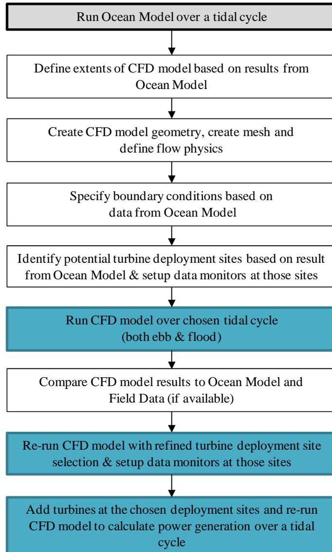
Figure 7-4: Flow chart of mid-field cross coupling approach
