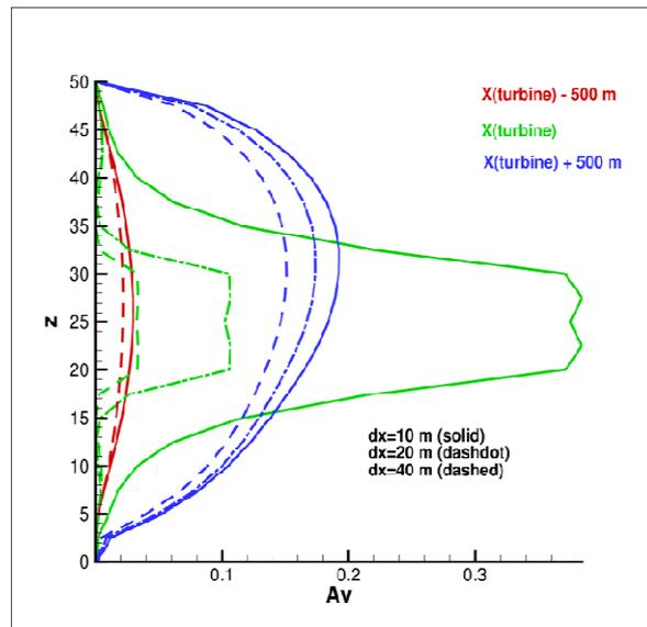
Figure 5-2: Vertical eddy viscosity using  $k-\epsilon$  turbulence closure.
