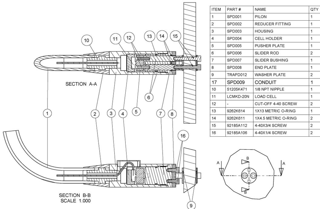
Figure 3-4: Detail of the load cell housing
