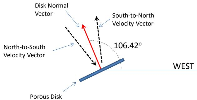
Figure 7-18: Turbine disk orientation for Petit Passage Model
