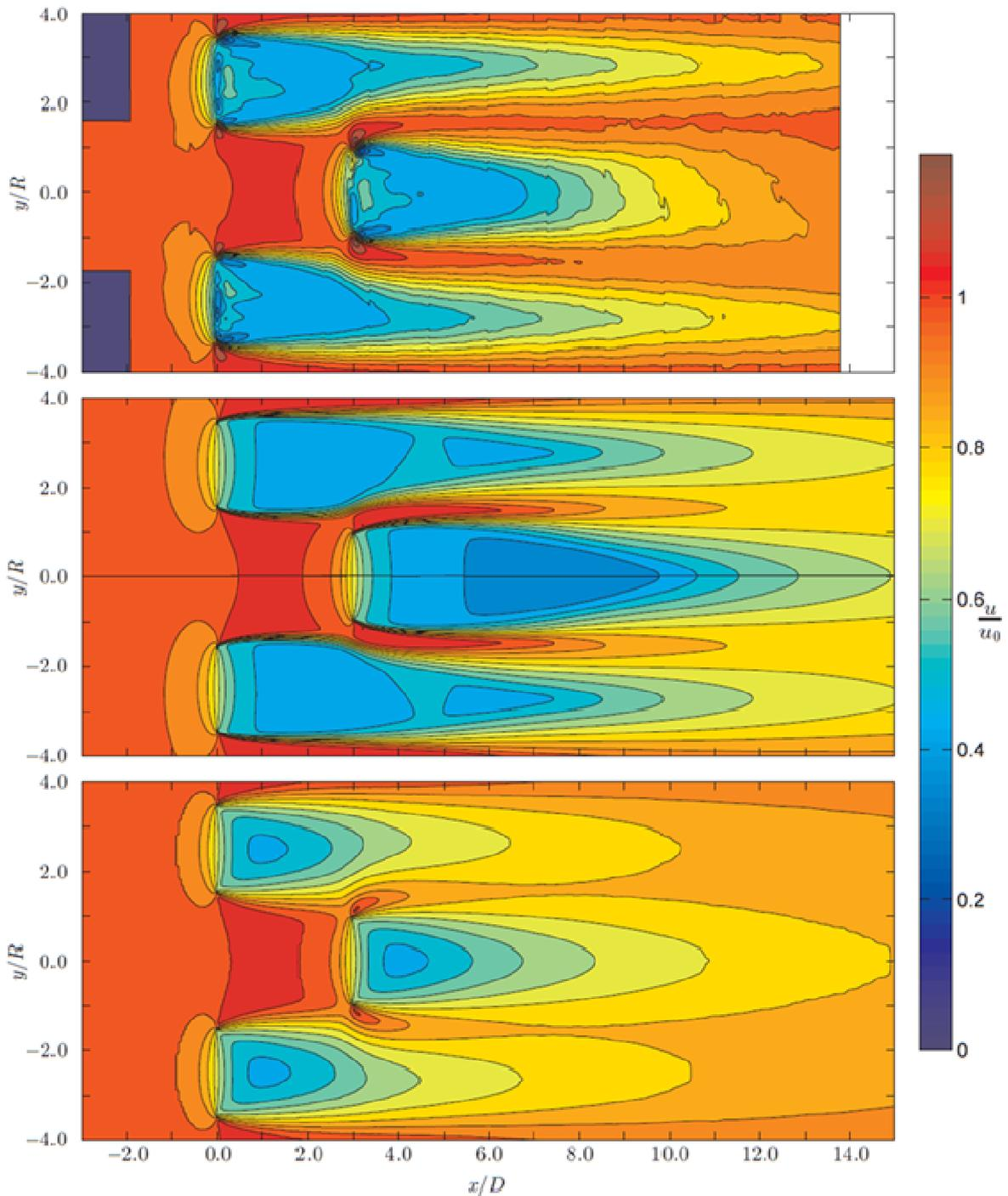
Figure 4-17: Contour plots comparing the wake structure for case 7b (three discs staggered) from PIV (top), UVIC sim (middle) and Mavi sim (bottom)
