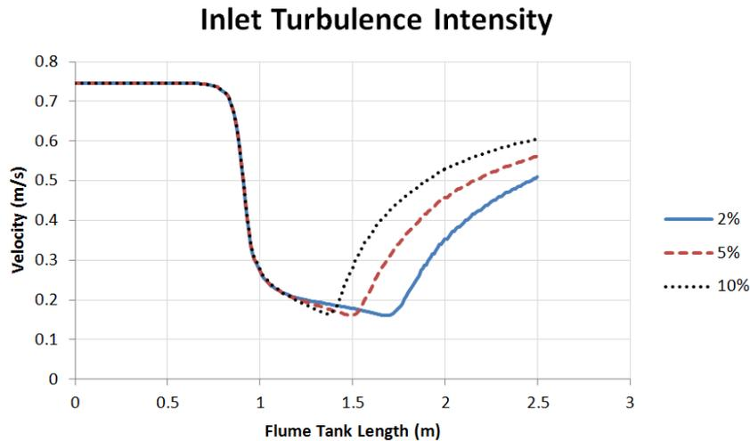
Figure 4-9: Centre-line velocity at different inlet turbulent intensities
