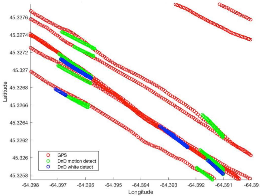
Figure 18: Minas Passage - Location comparison for GPS drifters to Drones and Drifters using aerial observations of GPS drifters. Shows good agreement with and without focusing on the white colour of the drifters.
