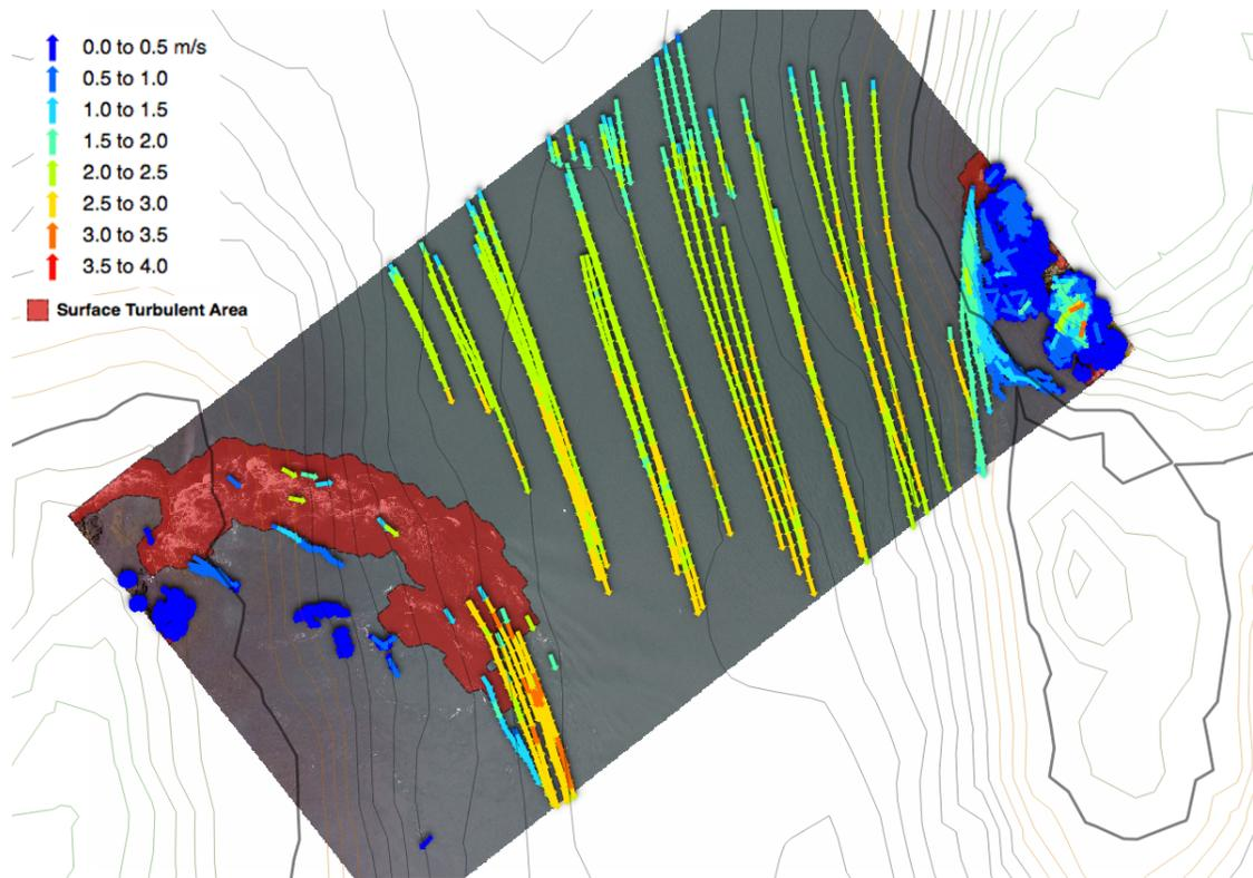
Figure 15: Grand Passage small channel - Surface turbulent areas and flow speeds calculated by Drones and Drifters using aerial observations of drifting pumpkins (north up). Long tracks down the main channel are from pumpkins. Flow speeds calculated near the eastern and western boundaries are from bubbles generated in turbulent areas. The experiment was conducted near the start of ebb tide with the water level above mean sea level (solid black bathymetry line).
