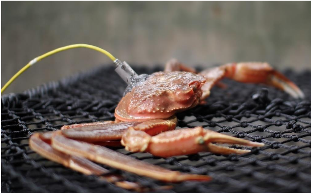
Figure 24 Heart rate bracket mounted with sensor on Snow Crab
