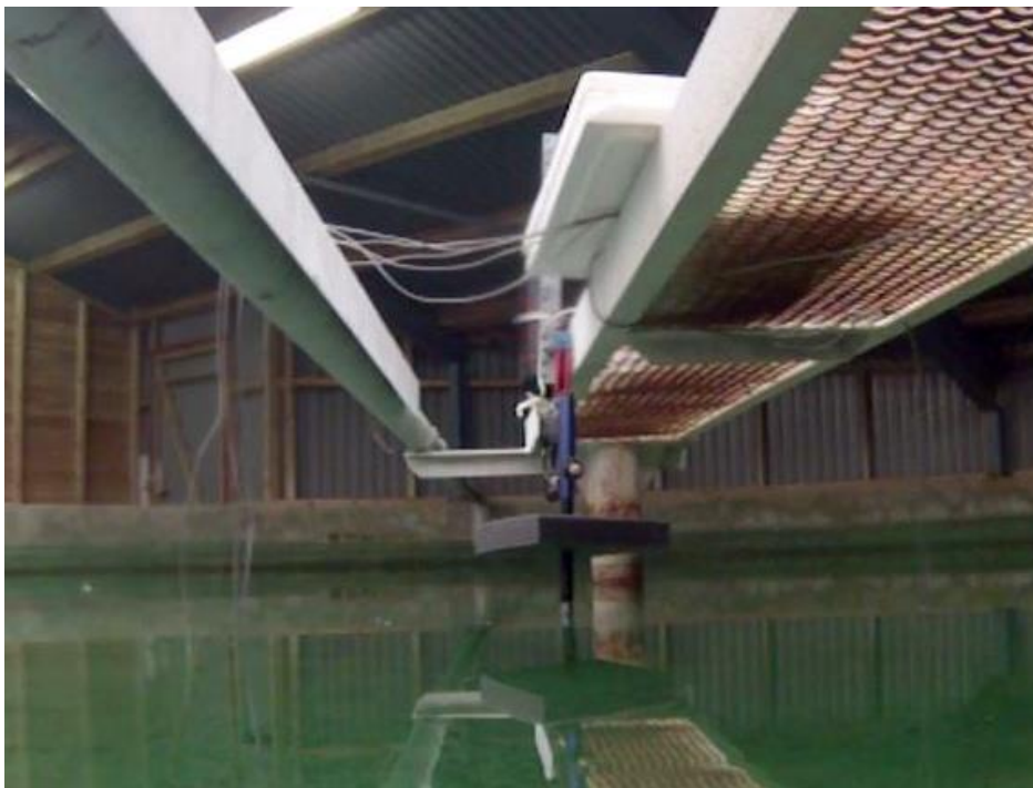
Figure 14 The air gun was placed in the centre of the testing tank containing the crab and mussel biosensors.
