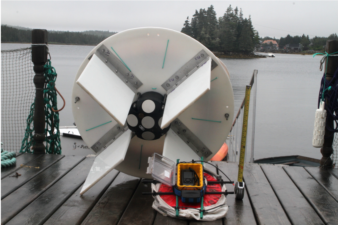
Figure 2: ADCP drifter and surface flow drifter - View 2
