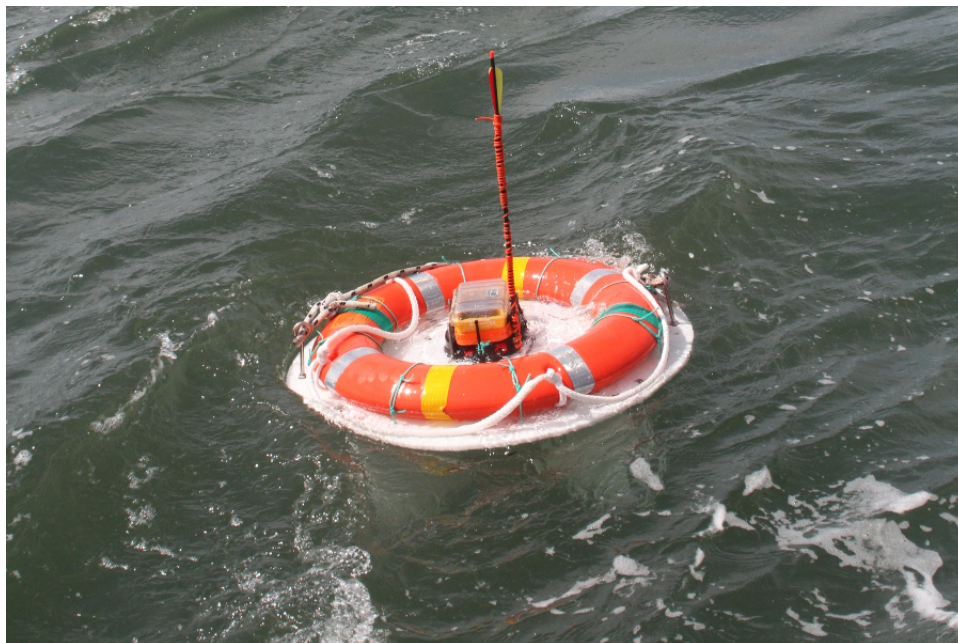
Figure 16: ADCP drifter in Minas Passage (near Cape Split)
