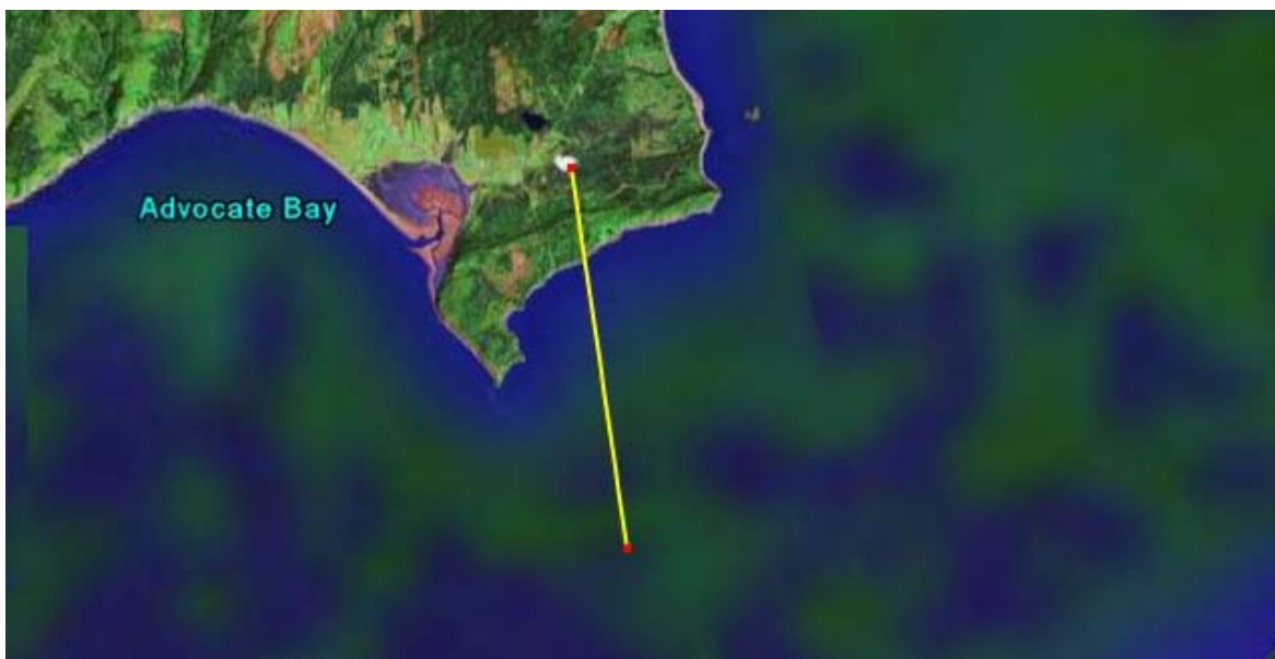
Figure 5.2-7 Distance from Site to Closest 12 kV Distribution Line for Nominal 500 kW Plant (8km, less if site is closer to shore)
