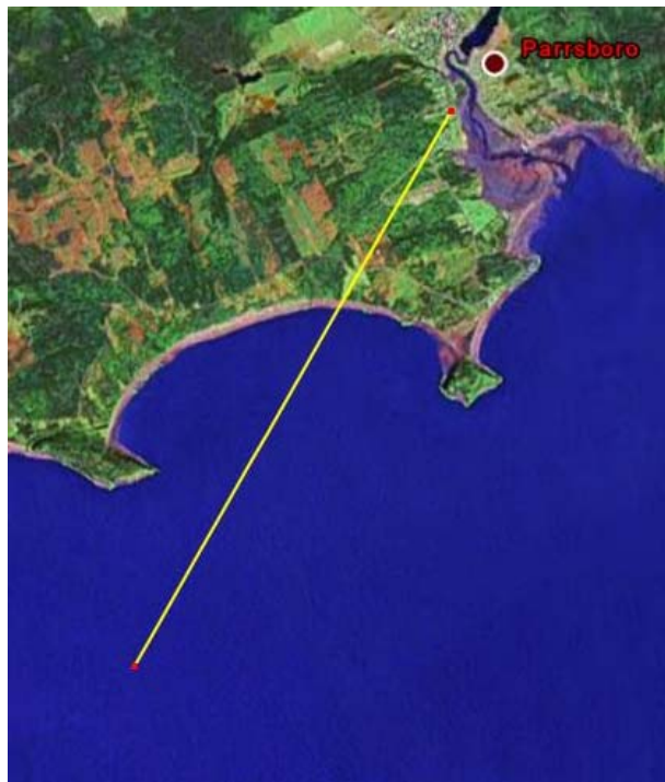
Figure 5.3-6 Distance from Site to closest 25 kV connection
