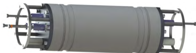
Figure 1. The Autonomous Multichannel Acoustic Recorder (AMAR; JASCO) used to measure underwater sound on one of the drifters.
