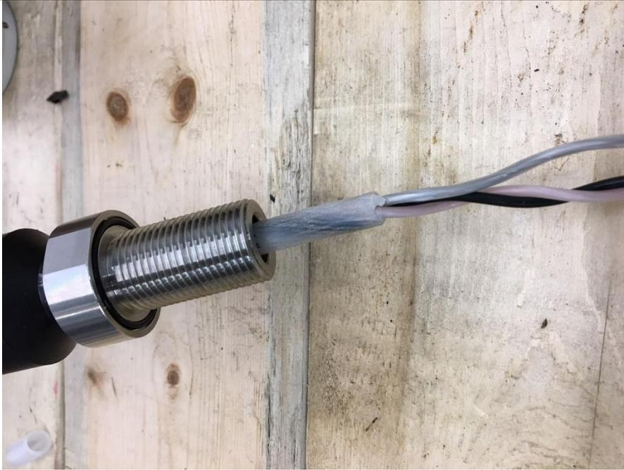
4. Fibre break out kit installed on stainless tube.
