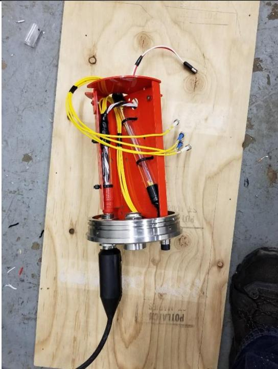
11. End cap and fibre bracket to be inserted in term can ensuring no kinks occurring.
