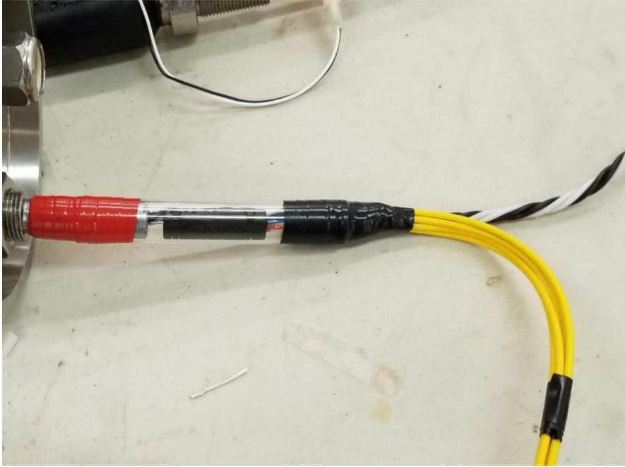
8. Completing fusion splices. Connector ends pre-inserted into additional section of 3/8" tubing. This will house the splices following fusing.
