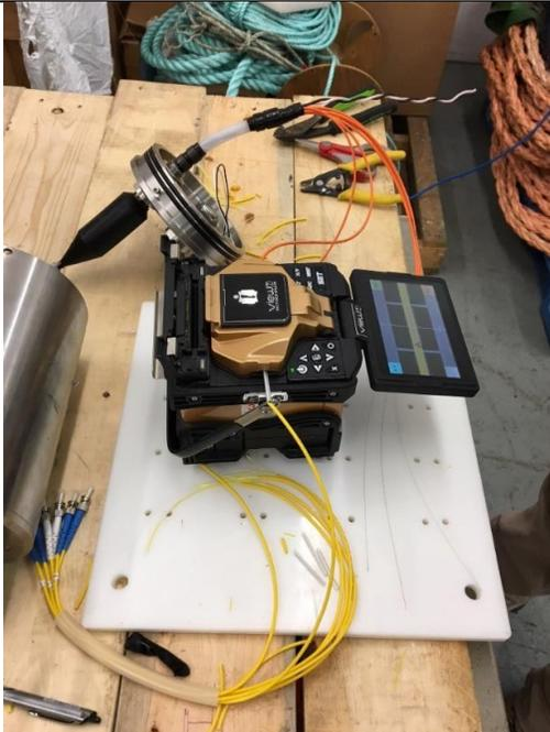
9. Three finished penetrator ends. Completed fusion splices in secondary acrylic tubing, with loose ST fibre connectors branching out.
