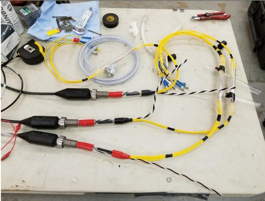
10. Penetrator fed through term can end cap and fixed to fibre bracket.
