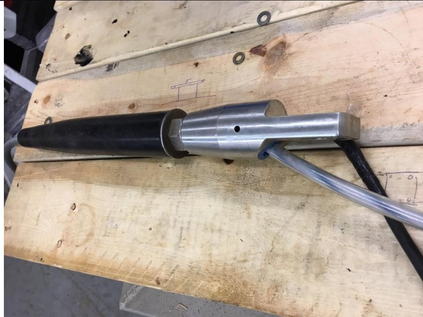
2. Water blocked penetrator to be installed on term can end.
