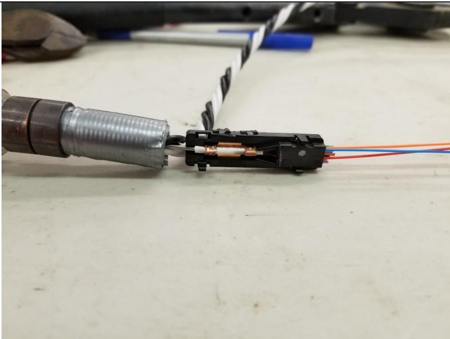
5. Inside fibre break out kit. White shrink tubing inserted inside stainless tube to mitigate chafing and fibre breakage.
