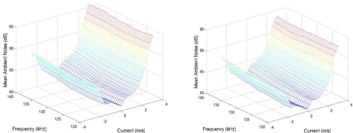
Figure 4.10. *icListenHF* hydrophone measures of mean ambient noise (dB) at 120-140 kHz, as a function of current speed (m/s), at location W1 during 6 June - 11 June 2014. **Left:** hydrophone 1211 without a foam shroud; **Right:** hydrophone 1239 with ½ inch, 20 ppi acoustic foam shroud.
