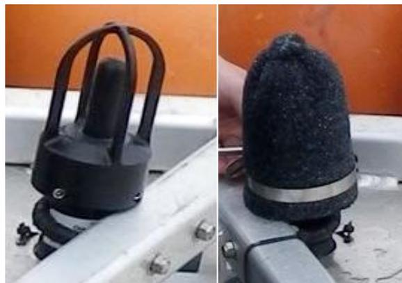
Figure 3.2. IcListenHF hydrophone tip with custom made HDPE guard (left) and with a ½ inch 20 ppi foam cover secured over the guard (right).
