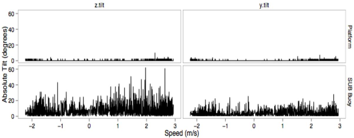
Figure 4.5. Tilt plots comparing pitch (z.tilt) and roll (y.tilt) with depth-averaged current speed (m/s) on the ebb (-) and flood (+) tides for the instrument platform and a SUB buoy located at station location W1.
