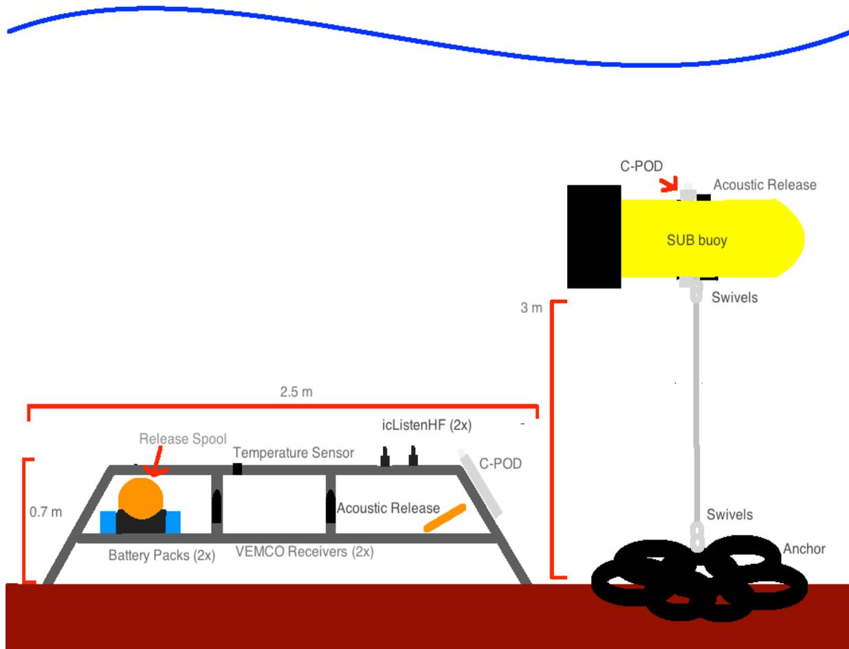
Figure 4.1. Mooring designs. **Left:** Instrument platform housing two icListenHF hydrophones with battery packs, a C-POD, and an acoustic release, plus other sensors (temperature, VEMCO receivers). **Right:** SUB buoy housing an acoustic release and a C-POD, and attached to anchor weight (about 200 kg) with a 3 m long riser chain.
