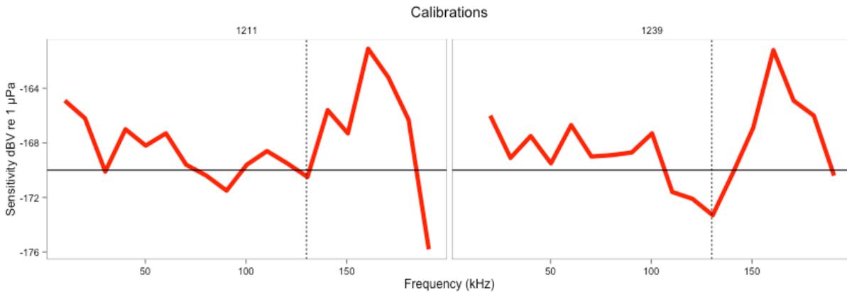
Figure 3.1. Calibration results for icListenHF 1211 and 1239 fitted with HDPE guards. Horizontal bar is a reference at -170 dBV re 1 $\mu$ Pa. Vertical dashed line (130 kHz) is within the frequency that harbour porpoises use for echolocation.
