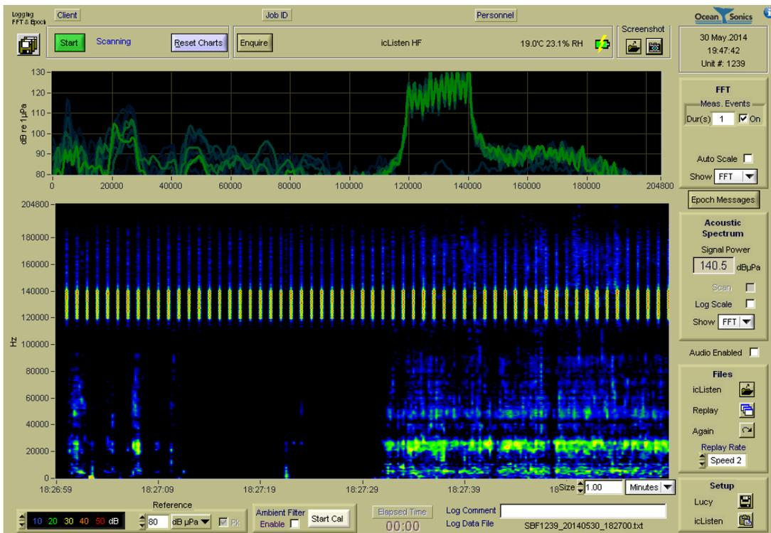
Figure 3.4 IcListen spectrograms from tank test trials. **Top:** without acoustic foam. **Bottom:** 1/2 inch thick, 20 ppi acoustic foam. The tank test trial commenced half way through the minute.
