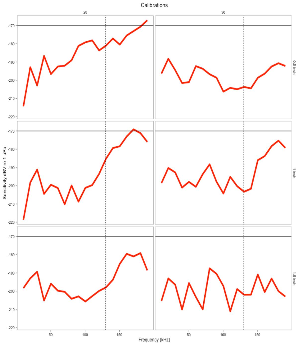
Figure 3.3. Calibration results for icListenHF 1239 for various shroud setups. Horizontal bar is a reference at -170 dBV re 1 $\mu$ Pa. Vertical dashed line (130 kHz) is within the frequency that porpoises use for echolocation. Rows represent various acoustic foam thicknesses tested and columns represented pore density (20 ppi and 30 ppi).
