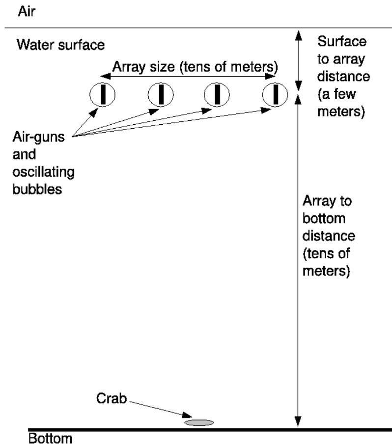
Figure 1: Typical configuration of array and crab that we are examining. The crab is assumed to be below the array, in tens of meters of water. The array is assumed to have multiple guns and to be spread over an area tens of meters on a side.
