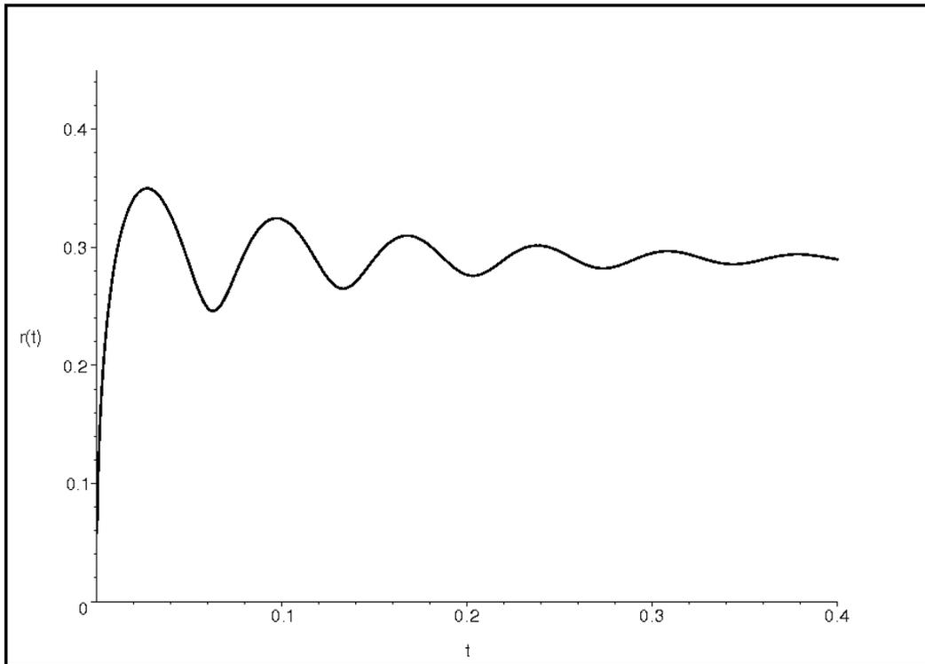
Figure 3: A typical radius vs. time for the bubble due to an airgun. This solution was found for a “GI” gun with 45 cu. in. generator chamber, 105 cu. in. injector chamber at a depth of 10 m.
