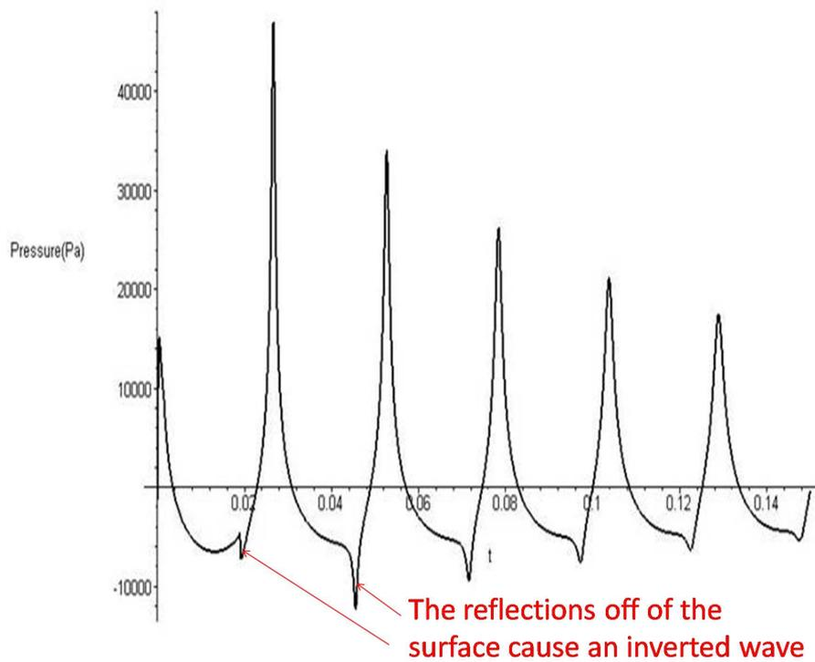
Figure 4: A typical pressure vs. time far from a bubble. This was found for a “GI” gun with 45 cu. in. generator chamber, 45 cu. in. injector chamber at a depth of 6 m and was calculated at a distance of 1 m from the air-gun. As noted, the effect of reflection off of the water surface was included in the calculation.
