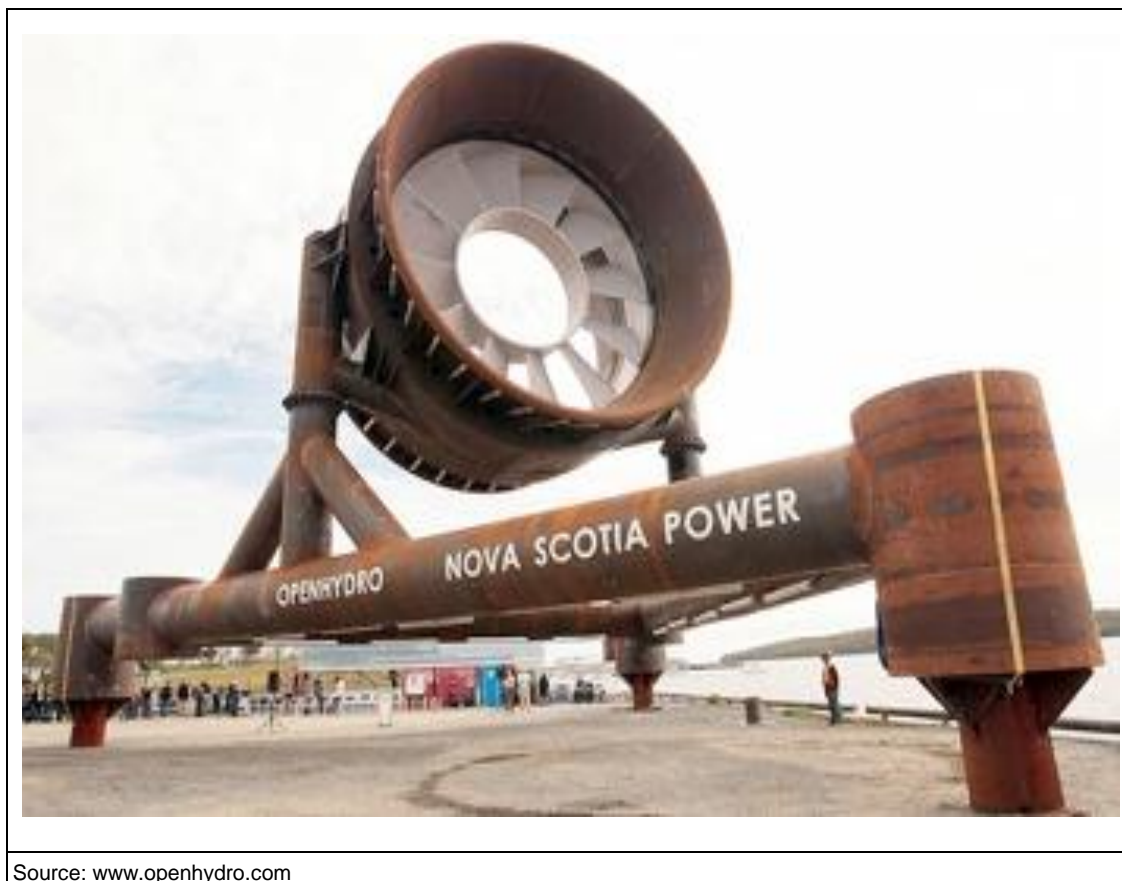
Figure 9. OpenHydro Technology (Horizontal Axis)
