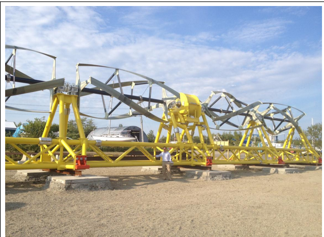
Figure 10. TidGen™ Technology (Horizontal Axis)
