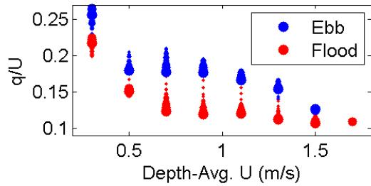
**Figure 3.** RMS turbulence intensity  $q$ , normalized by the depth-averaged mean speed  $U$ , vs.  $U$ , for heights between 2.1 and 10.1 m. Symbol size increases with height.
