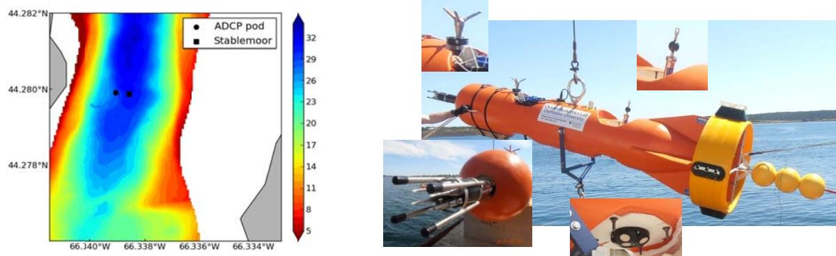
**Figure 4.** Left: Bathymetry in Grand Passage and the locations of the ADCP bottom pod and Stablemoor buoy. Right: The Stablemoor buoy and associated instruments during the 2<sup>nd</sup> week of the 2013 experiment: clockwise from lower left, the RSI Microrider in the nose, with 4 shear probes and the probe guard; a Nortek Vector single-point acoustic Doppler velocimeter; a JFE single-point electromagnetic flowmeter; and a downward-looking Nortek bottom-tracking AD2CP.
