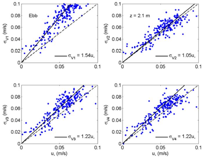
**Figure 1.** RMS beam velocities vs  $u_*$ . The solid lines indicate the expected relationship based on laboratory and atmospheric boundary layer measurements. The dashed line is the 1:1 line.
