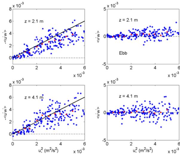
**Figure 2.** Reynolds stresses vs friction velocity squared at two different heights above bottom. The panels at left show the along-channel Reynolds stress, with the solid line indicating 1:1. The panels at right are the cross-channel Reynolds stress estimates, the dashed line indicating zero.
