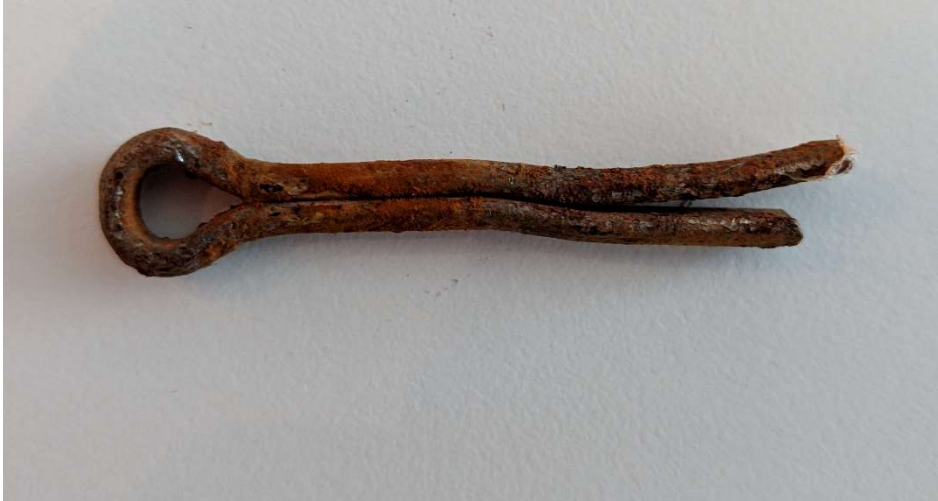
Figure 25 - Cotter pin used in safety shackle. Zinc plating is entirely lost and severe corrosion can be seen.
