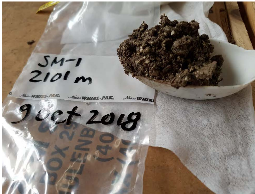
Figure 10. Cuttings samples collected from the SM-1 well: a) 2086 m, note fibrous material and white plastic; b) 2101 m, stained with heavy oil.
