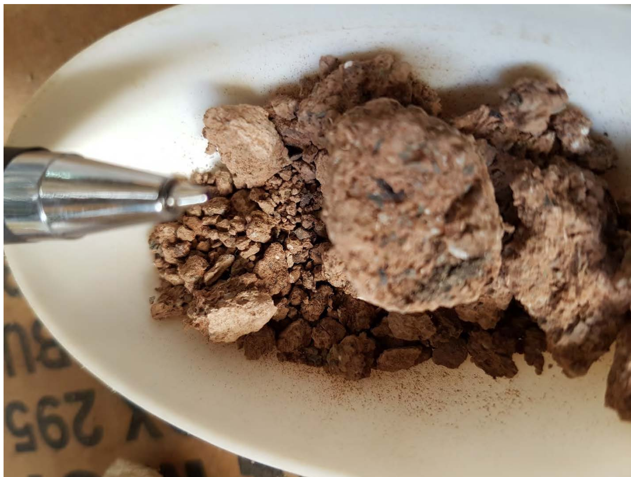
Figure 13. Cuttings samples from 3360-3370 m collected for extraction to investigate if there was oil staining. Note black blobs within the red sandstone.
