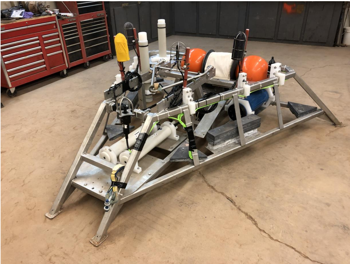
Figure 1 PAM instrumentation mounted on the FORCE lander.
