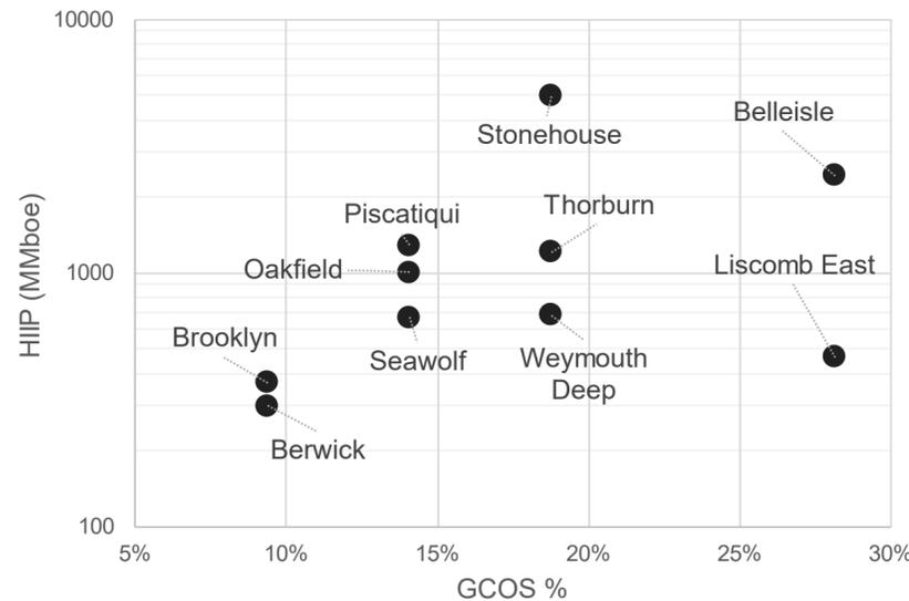
Figure 3: Top 10 leads hydrocarbon in place (unrisks) versus geologic chance of success
